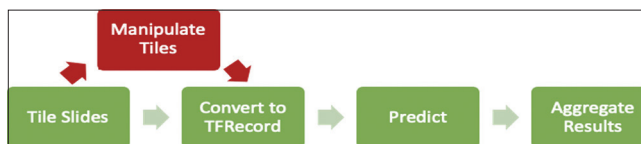
Figure 2: Schematic of processing steps undertaken by our Snakemake workflow. The “manipulate” tiles step in red was only applied to experimental studies
